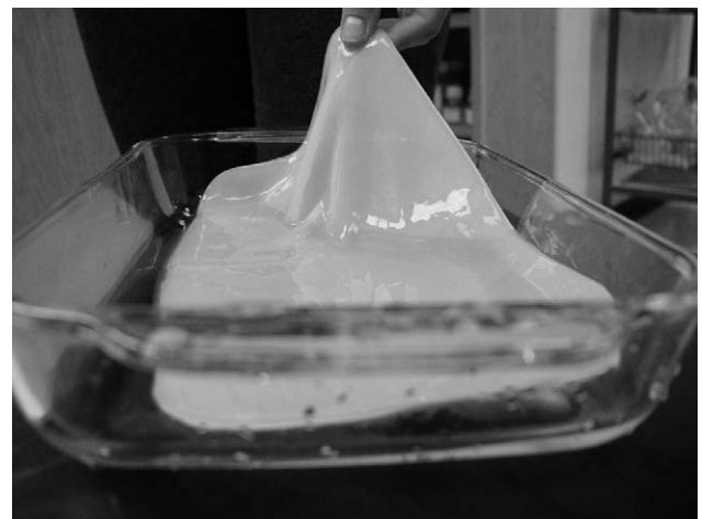
Fig. 2. The never-dried microbial cellulose membrane is a non-pyrogenic and fully biocompatible biomaterial with high mechanical strength.
